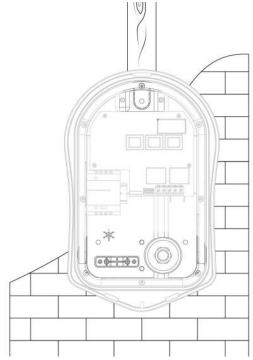
Using zappi template mark mounting holes. Use top and 2 bottom holes left/right for brick use 2 vertical holes if mounting to a stud wall or joist. 6
