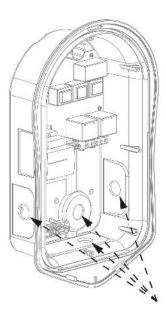
Remove all 8 screws from the enclosure and carefully lift away.
