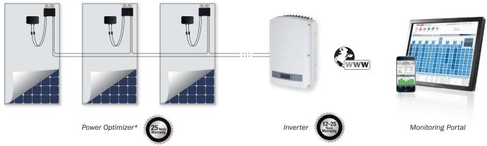
\* SolarEdge power optimizers can operate with any inverter.
